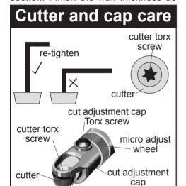
Tighten the cutter torx screw using only the key as shown above. To remove the cut adjustment cap first remove the cutter and slide the cap away.
