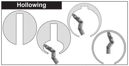
Drill a central bore to remove the slow moving centre section and allow waste material from the hollowing tool to clear from the cutting area. After creating the centre bore, begin hollowing the first section. Finish the wall thickness as
