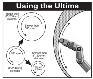
The Ultima is designed to cut with little effort. Use with a smooth sweeping action to give a comfortable and controlled cut.
