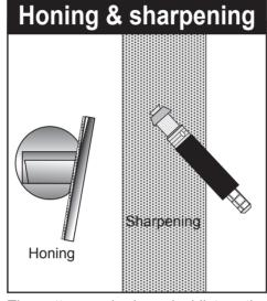
The cutter can be honed whilst on the tool using a diamond or honing stone. Gently sweep around the face keeping the abrasive flat on the bevel.
