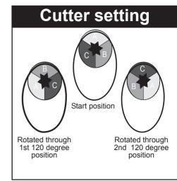
When the cutter becomes less sharp it can be rotated through 120 degrees to reveal a new sharp edge. This can be done twice before sharpening is required. Always clear dust from Allen & Torx key sockets.
