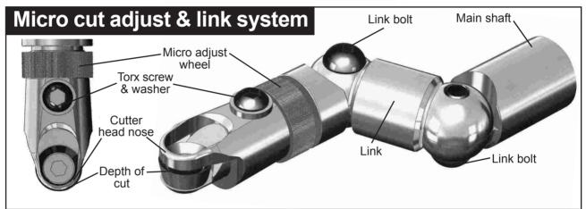
The depth of cut can be altered depending on the type of wood being used, whether it is wet or dry and the speed of the lathe. The depth is determined by the amount that the cutter is protruding from the nose of the cutter head. This distance is factory set slightly wider than the thickness of paper but less than that of a credit card. The depth of cut is the thickness of waste material that will be removed during each cut.
